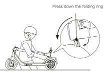
Hold the stem and pull the folding ring, attach the hook to the locking clip on the side of the mudguard.
