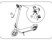
Place the brake lever on the handlebar, tighten it firmly with hex wrench to be sure it won't loosen.
