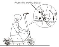
Power off the scooter, hold the stem, press the locking button and pull the lever, bend the handlebar stem towards the footrest.
