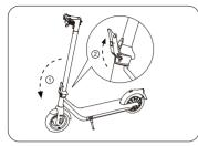
Unfold the stem and fasten the folding wrench. Make sure the Unlock key springs up normally after fastening. Be sure to buckle up properly.
