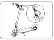
Install the handles on the stem and firmly tighten it according to the correct position and direction marked on the label.
