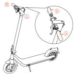
4. Install the handles on the stem and firmly tighten it according to the correct position and direction marked on the label.
